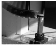
Side load impact tests show that the Rain Bird 7005 and 8005 rotors are stronger than the competition. The 7005 and 8005 rotors consistently withstood the maximum impact force of the test equipment.
